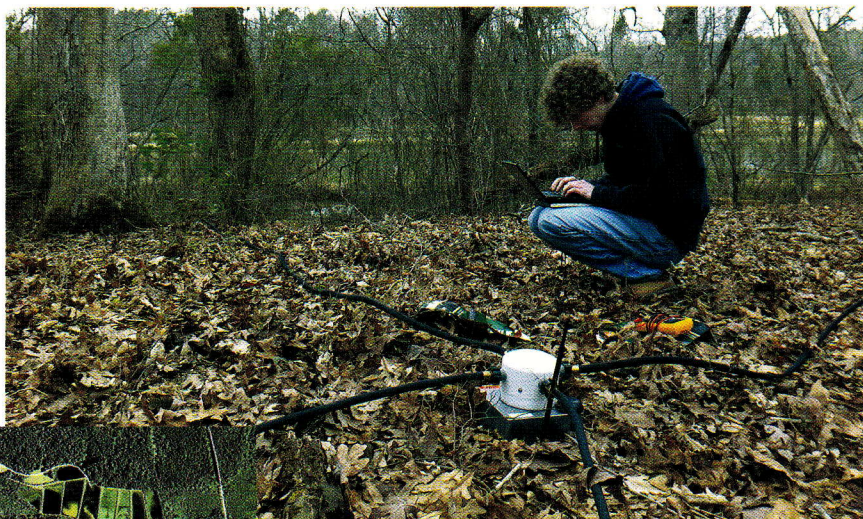
Setting up infrasound sensor at the Field Station
